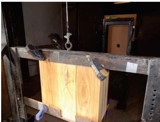
Figure 4: CLT tile mounted in steel frame for ballistic testing viewed from back, non-strike face (foreground) and looking toward velocity screen (background).
