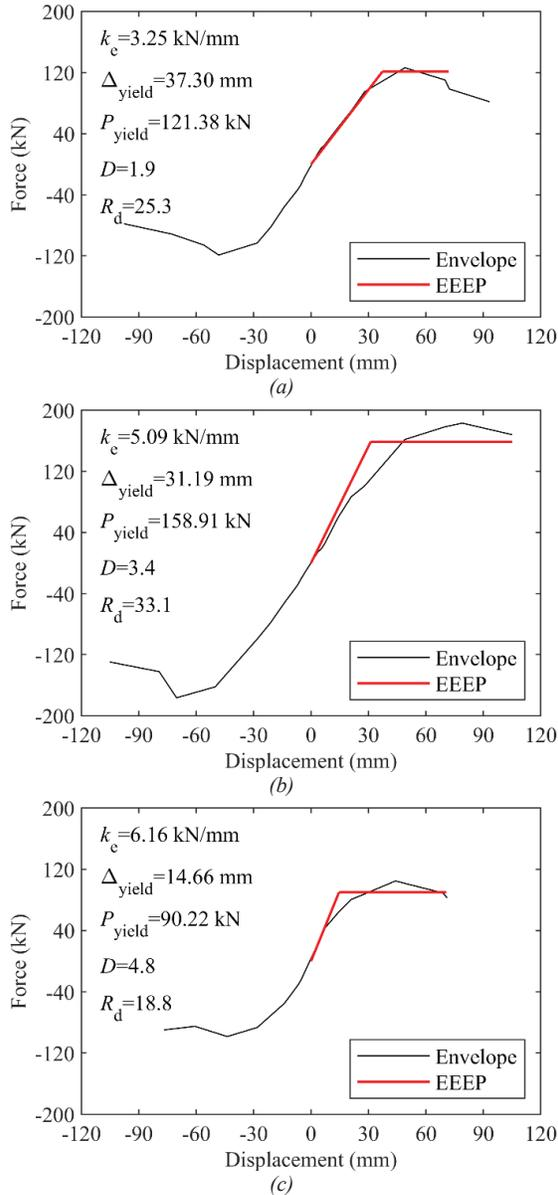
**Figure 7:** EEEP analysis result of (a) group A-V, (b) group B-V, and (c) group A-H.
