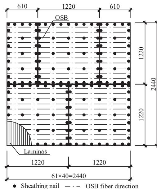
**Figure 1:** Dimensions (in mm) of tested group A-V.
