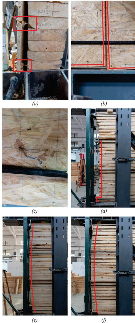
**Figure 6:** Failure modes of (a) sheathing nail embedment, (b) sheathing dislocation, (c) sheathing nail withdraw, (d) lamina nail failure, (e) floor shear and flexural combined deformation of relatively larger sheathing nail spacing (group A-V), and (f) floor shear deformation of relatively smaller sheathing nail spacing (group B-V).
