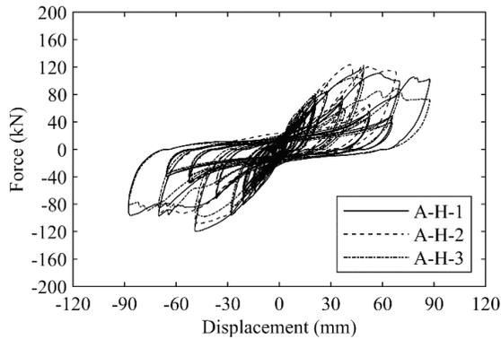
**Figure 5:** Hysteresis loops of (a) group A-H, (b) group B-V, and (c) group A-V.
