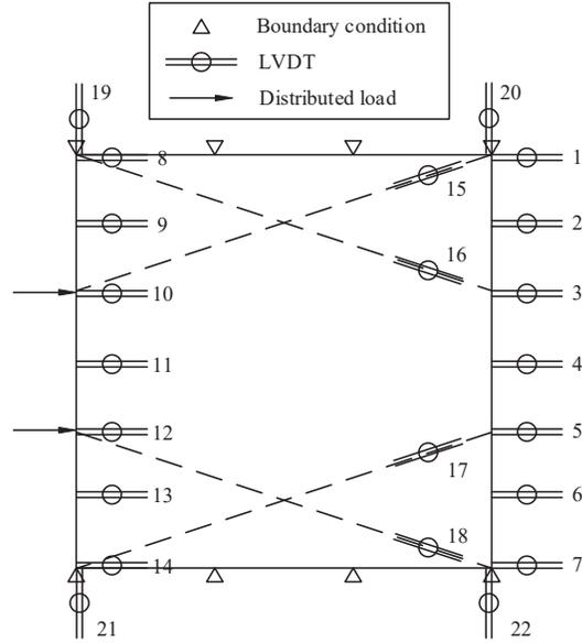
Figure 4: Layout of LVDTs.
