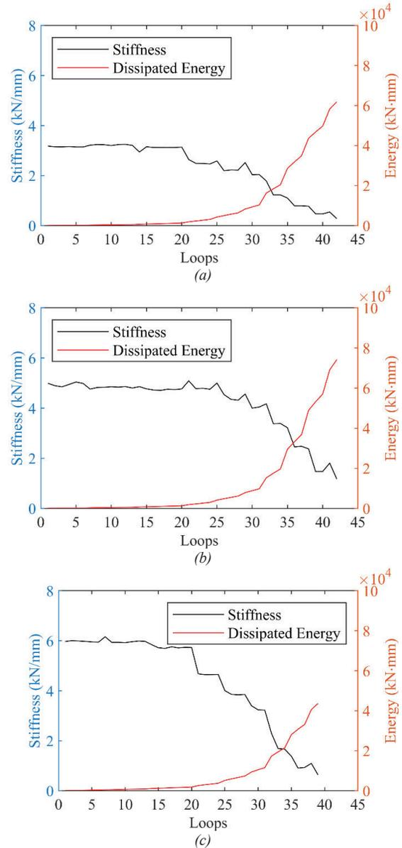
**Figure 8:** Secant stiffness and cumulative dissipated energy per hysteresis loop of (a) group A-V, (b) group B-V, and (c) group A-H.
