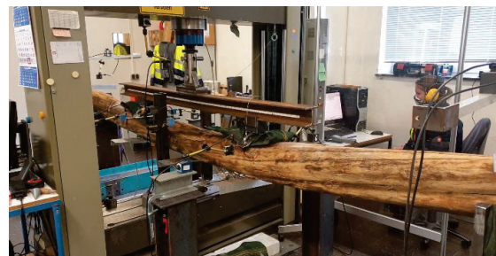
Figure 2: Natural and load-induced distortion of test specimen.
