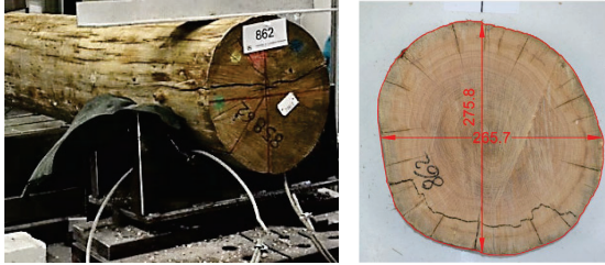
Moment of inertia X: 292,666,326 mm 4 Area: 59,384.48 mm 2 Moment of inertia Y: 272,328,664 mm 4 Circumference: 883.73 mm
