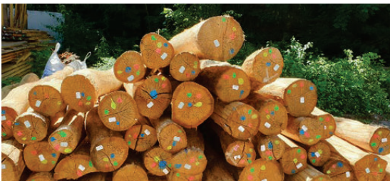
Figure 1: Debarked small-diameter oak logs for testing.
