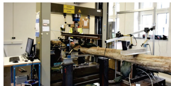
Figure 4: Standard test arrangement with span-to-depth ratio 18:1 [7]; DiShape surface model of log no. 862 and lab view on log no. 862 waiting for action.
