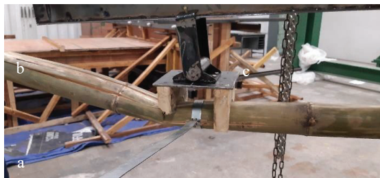
Figure 6: Failures due to bending test on the construction site
