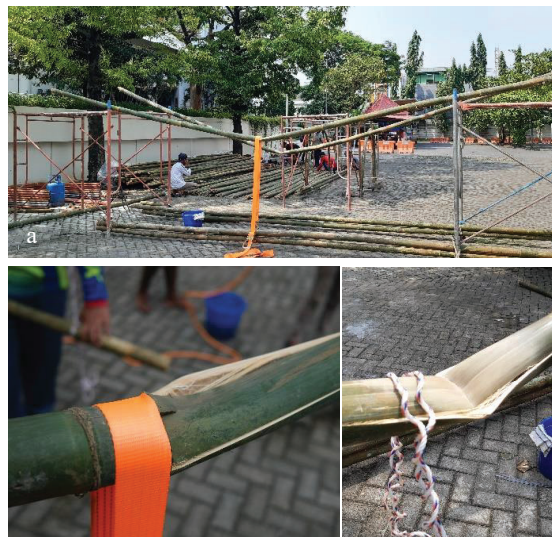
Figure 6: Failures due to bending test on the construction site
