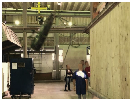
Figure 5: Soft body impact test in progress. The picture shows the moment after the leather bag is abandoned.
