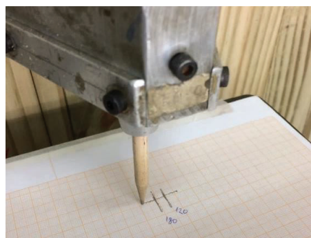
Figure 6: Soft body impact test in progress. The picture shows the measurement of the instantaneous horizontal displacement (dh) and the residual horizontal displacement (dhr) of the panel by the depth calliper.
