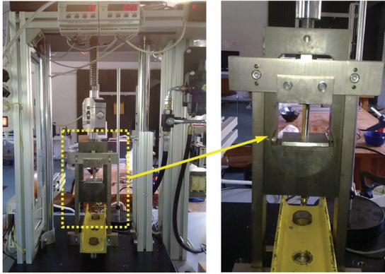
Figure 2: Compression test setup
