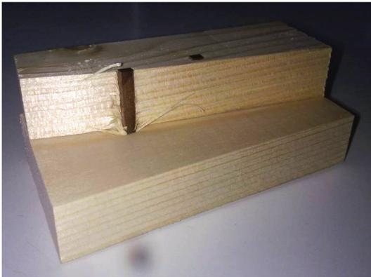
**Figure 6.** Wooden nails joining two pieces of spruce wood.
