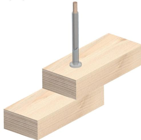
**Figure 8.** Concept for the assist tool for avoid buckling during nailing.
