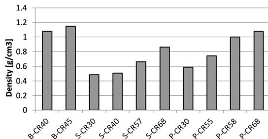
Figure 3: Density of densified specimens
