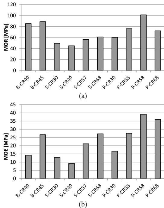
Figure 4: Mechanical properties of densified specimens measured during compression test (a), modulus of rupture (MOR)(b), modulus of elasticity (MOE)
