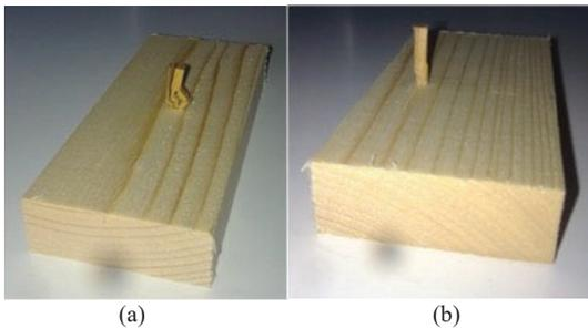
**Figure 7:** Typical damages to the wooden nail occurring during insertion; (a) splitting of the nail, (b) collapse of the wood fibre due to excessive compression stress.
