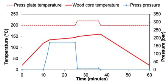
Figure 1: Schedule of thermo-hydro-mechanical (THM) densification.
