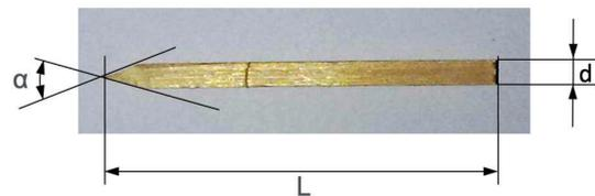
Figure 5: Image of the developed wooden nail and recommendations for its design.
