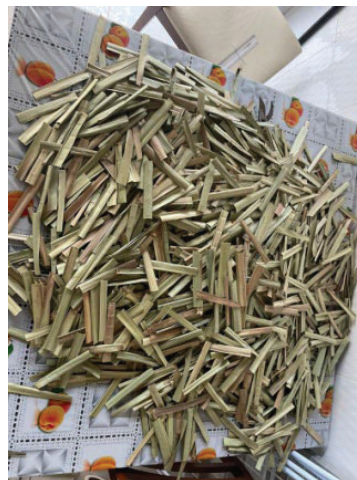
Figure 6: Material cut into 14 cm sheets and natural leaf width of approximately 4 cm. (Source: Author)
