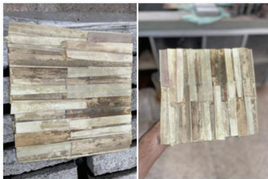
Figure 7: Samples of completed babassu leaf fiber boards.
