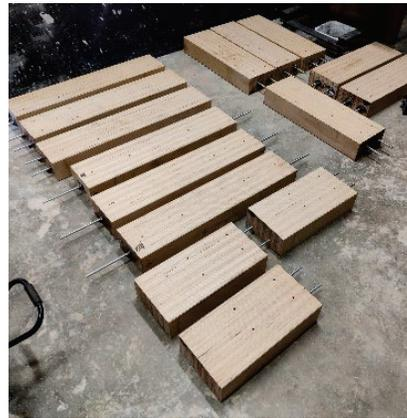
Figure 7: Specimens following the application of the adhesive.
