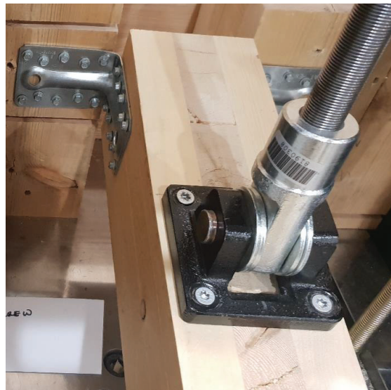
Figure 17: Experimental setup of CLT connection made of angle bracket ABR9020 and screws.
