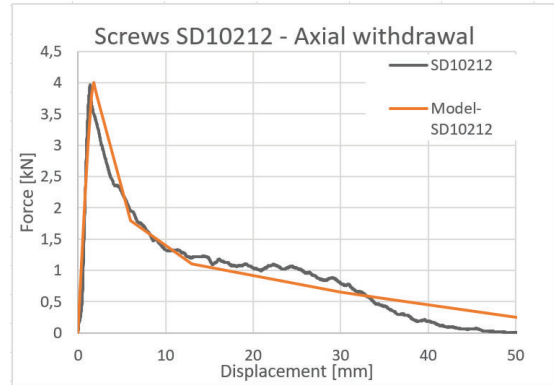
Figure 8: Results of numerical simulation of SD10212 screw in CLT connection compared to the numerical simulation.
