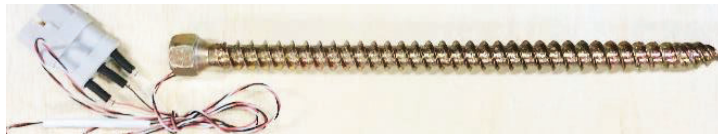
Figure 1: Self tapping screw with strain gauge
