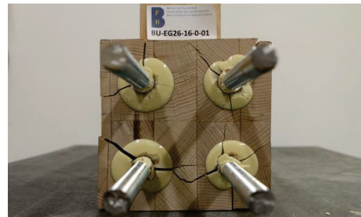
Figure 1: Typical BiR failure in beech glulam – wood splitting due to transverse tension without a recess in the bondline
