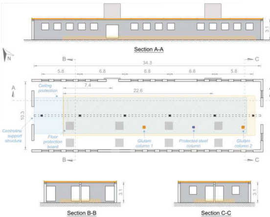
Figure 2: Floor plan and sections of the compartment used for the CodeRed experiments. Units in metres.
