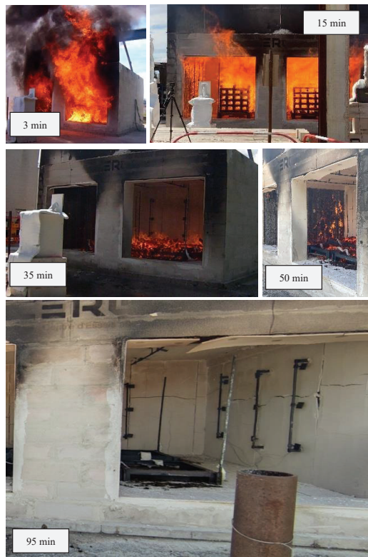
Figure 9. Test 3 stages: growth (1-upper left), steady-state (2-upper right), decay (3-lower left); Continuous combustion of the exposed wall (4-lower right); Cracks after burnout of the moveable fuel load (5- last).
