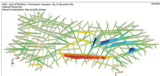
Figure 12: Moment diagram of the result beams
