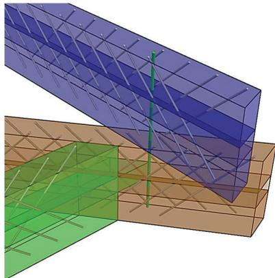
Figure 7: Illustration of a connection of three beams
