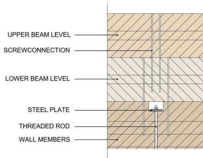
Figure 6: Anchorage detail
