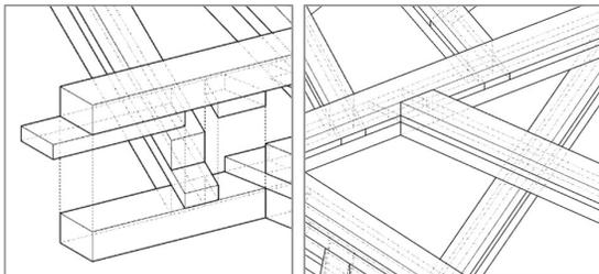
**Figure 16:** Intertwined beam layers
