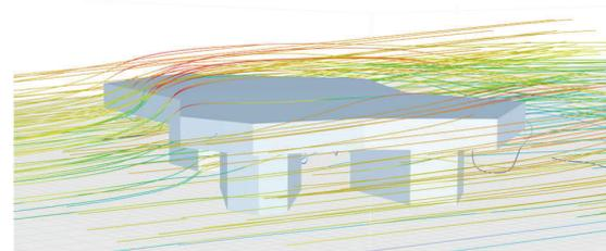
Figure 5: Extract from the FE-wind calculation
