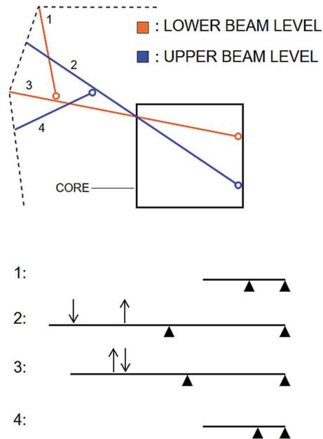
Figure 8: Illustration of the structural concept of the roof
