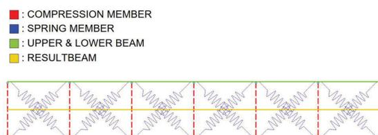
Figure 13: Illustration of a beam in the structural model
