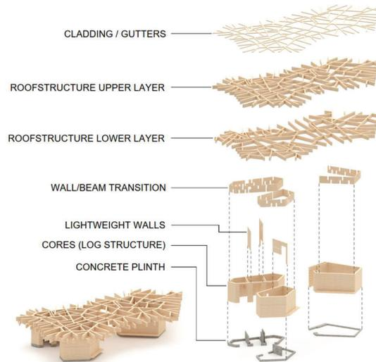
Figure 3: Illustration of the service building components by Atelier Oslo (translated)
