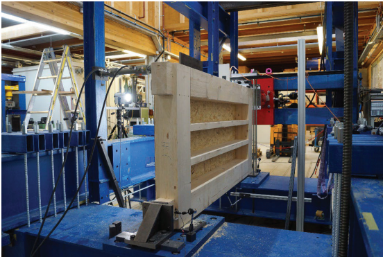
Figure 8: Timber-framed shear wall specimen mounted in the test rig and ready for investigation of the shear resistance of the OSB/3 panels applied as sheathing material.
