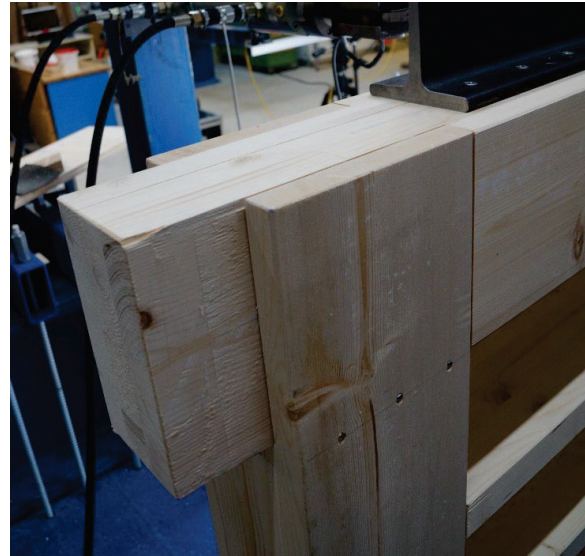
Figure 5: Construction detail of mortise and tenon joints at the corners of the tested timber-framed shear wall elements.
