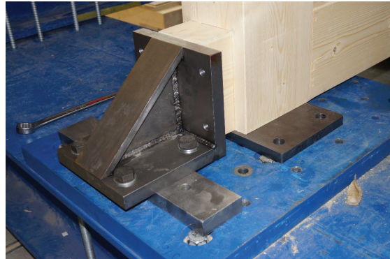
Figure 10: The horizontal reaction force was transferred to the test rig via a massive steel angle bracket. The vertical compressive force was transmitted through contact.
