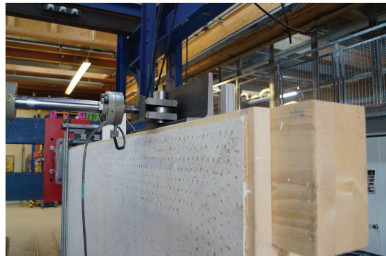
Figure 11: Tilting of the specimen was prevented by means of a 50 kN hydraulic jack maintaining the out-of-plane displacement on the top rail at a value of 0 mm.
