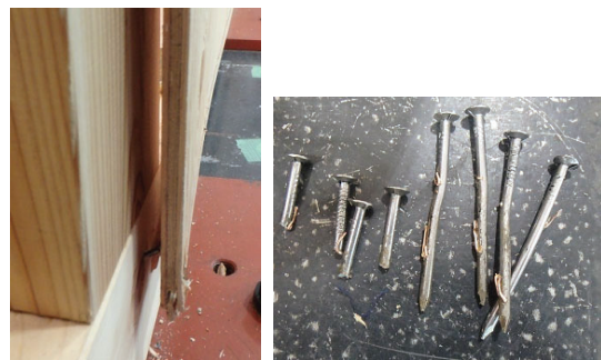
Figure 7: Plywood shear wall specimen and nails after the test
