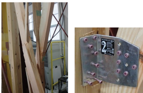
Figure 9: Braced shear wall specimen with conventional brace connectors after the test
