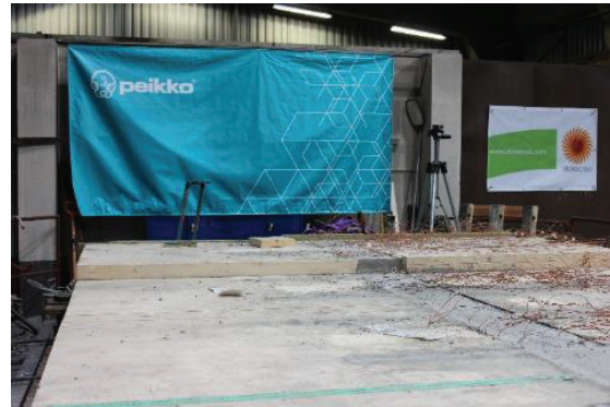
Figure 12: Specimen for the two-hour charring test without loading.
