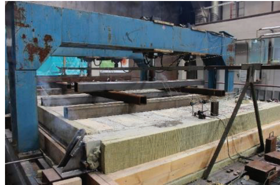
Figure 14: Specimen for the 90-minute loaded fire test consisting of two edge beams, an intermediate beam and two CLT panels.
