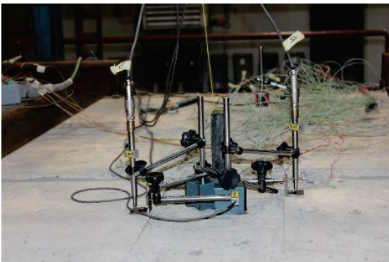
Figure 20: Assembled displacement sensor in the joint area at mid beam span in vertical and horizontal direction.
