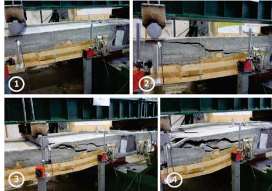
Figure 9: Concrete topping crack pattern development in composite timber slabs.
