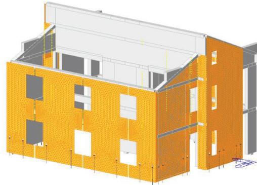
**Figure 10:** Finite Element Model of the retrofitted building
