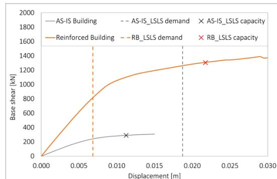
**Figure 11:** Comparison between the pushover curve of the As-is building and retrofitted building for the main direction
