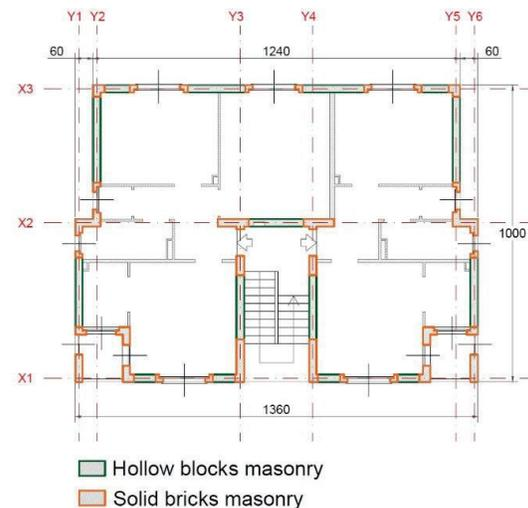
Figure 3: Floor plan of the building
