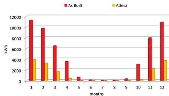
Figure 14: Comparison between the energy performances of the building in the as-is and retrofitted conditions
