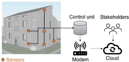
Figure 2: Structural Health Monitoring concept
