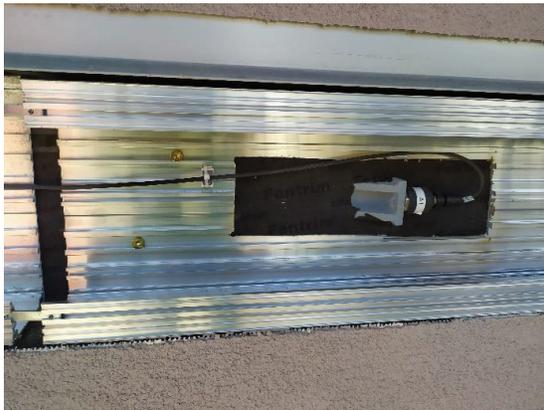
**Figure 15:** Placement of an accelerometer within the Fluxus system
