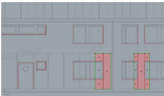
Figure 10: A screenshot from Grasshopper showing a first automatic element division on a façade in Lombolo.
