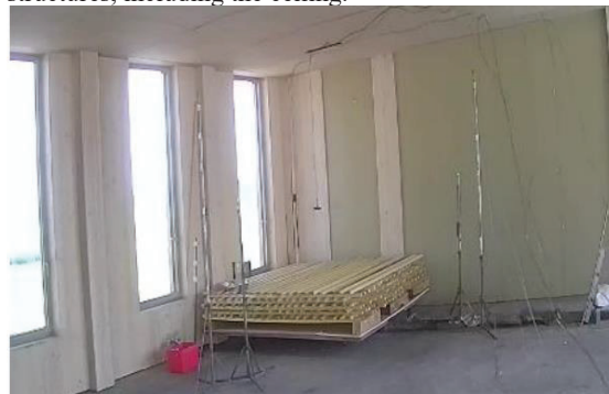
Figure 11: fire start at the end of the office floor
