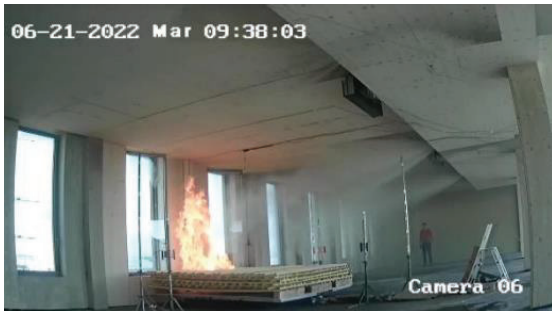
Figure 12: activation of water mist
