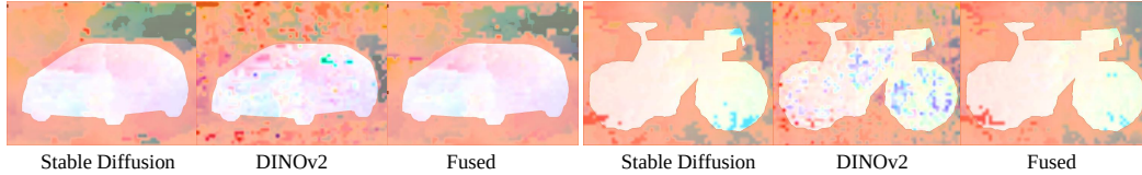
Figure 4: Semantic flow maps using different features. White mask indicates valid pixels and orange mask separates the background flow. SD features yield smoother flow fields versus DINOv2’s isolated outliers.
