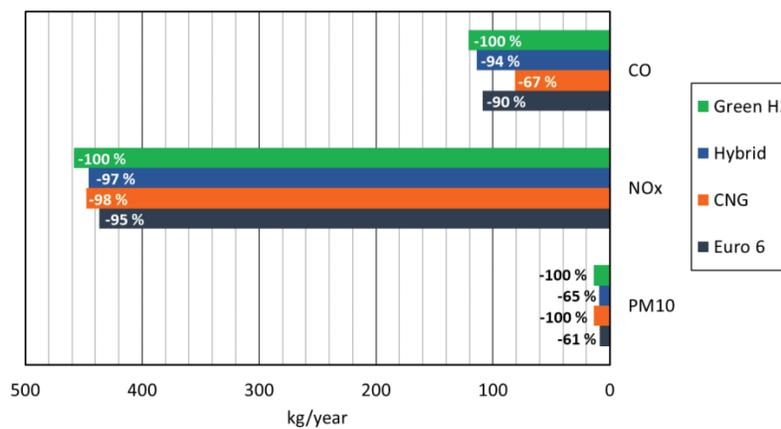
**Figure 4:** Pollutant emissions saved per Euro 3 diesel bus replaced. The percentage values indicate the reduction with respect to the Euro 3 scenario
