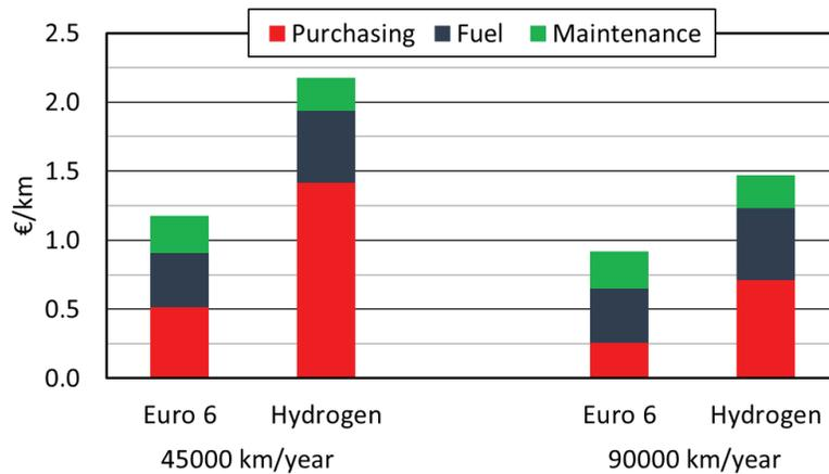
**Figure 5:** Diesel and hydrogen bus mileage cost, for 45'000 km/year (reference case) and 90'000 km/year
