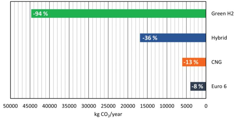
**Figure 3:** CO<sub>2</sub> saved per Euro 3 bus replaced. The percentage values indicate the reduction with respect to the Euro 3 scenario
