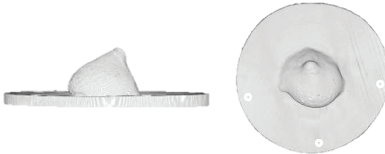
Figure 7. An example of an irregular geometry that has a region that could impact the body with a relatively high energy density.
