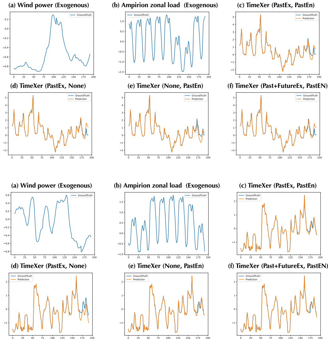
Figure 11: Two showcases (placed at the top and bottom respectively) of TimeXer in forecasting with exogenous variables from DE datasets. (a) and (b): The showcases of two exogenous variables Wind power and Ampirion zonal load. (c) The prediction results of TimeXer using the historical information of endogenous and exogenous variables. (d) and (e): The prediction results of TimeXer only use the historical information of exogenous or endogenous variables. (f) The prediction results of TimeXer using the historical information of endogenous and exogenous variables, and the future prediction values of exogenous variables.
