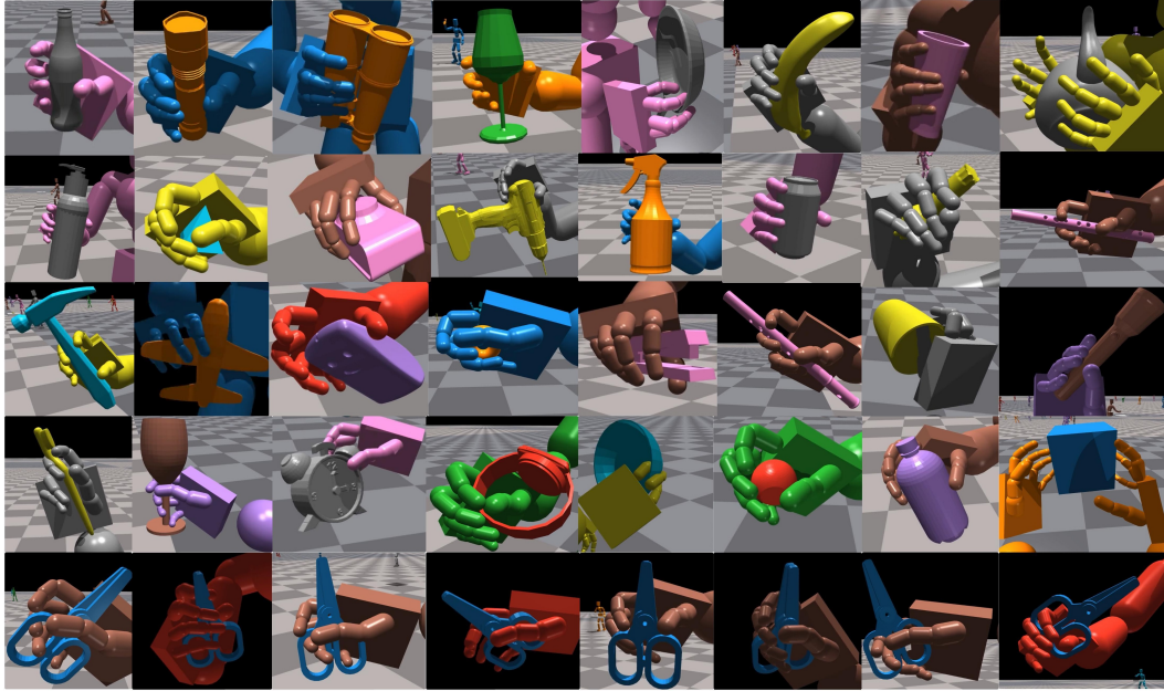
Figure 4: ( Top rows ): grasping different objects using both hands. ( Bottom ) diverse grasps on the same object.
