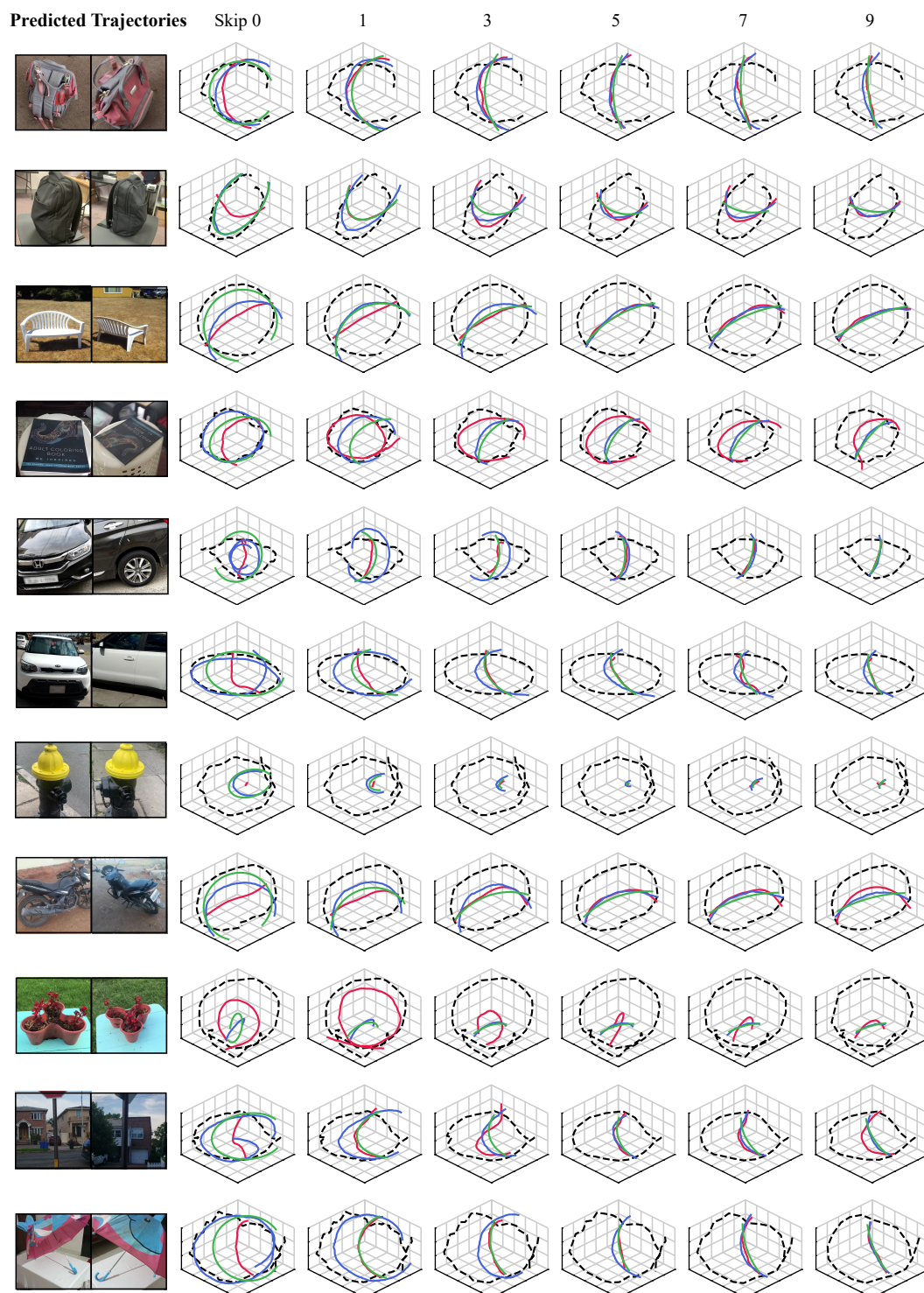
Figure 7: Failure Cases. Select failure cases. Interestingly, NIso appears to consistently fail when the background and foreground objects are respectively far from and close to the camera. In such cases, depth maps are often ill-defined, suggesting NIso may encourage models to reason about the underlying 3D structure of the scene.
