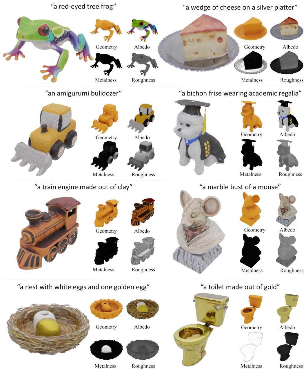
Figure 6: Text-to-3D meshes generated by Meta 3D AssetGen along with their PBR decomposition. Note that Meta 3D AssetGen provides detailed albedo and material properties, as highlighted by the metalness of the platter (top right) and the golden objects (last row).
