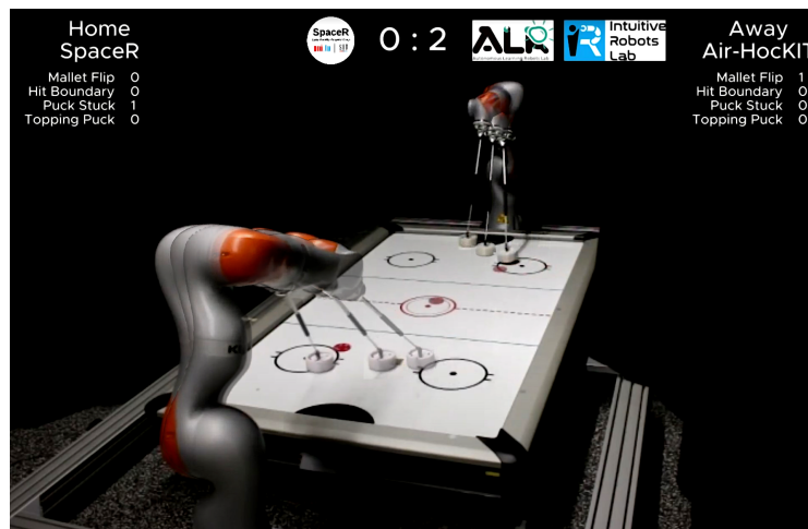
Figure 1: Game played in the real world between SpaceR and Air-HocKIT. The Air-HocKIT robot (back) hits the puck and the SpaceR robot (front) defends the attack to take control of the puck.
