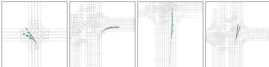
Figure 5: Qualitative results on V2X-Traj. There are several interesting cooperative scenarios at the challenging intersection, including speed-up, lane changing and turning. We visualize only the forecasting results of the target agent in each scenario for clarity. The ground-truth trajectories are shown in red, and the multimodal predicted trajectories are shown in green.
