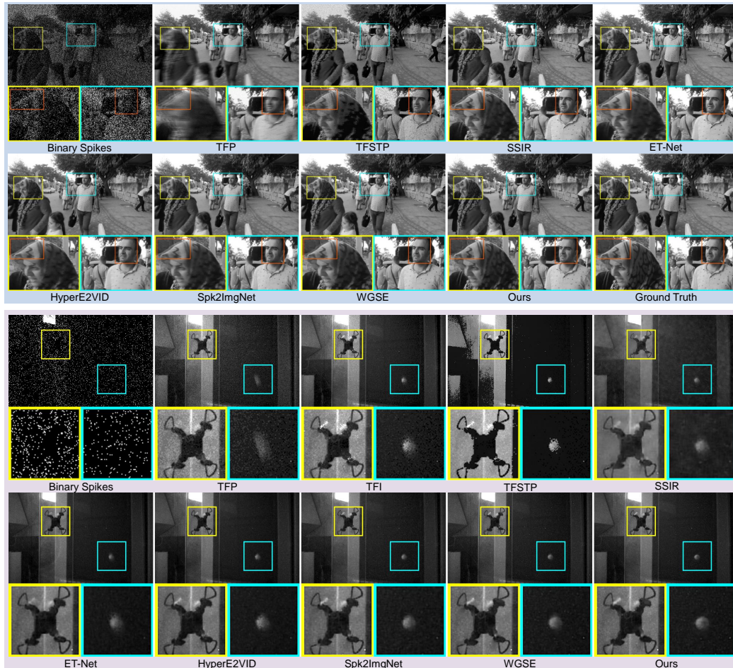
Figure 4: Visual comparison on synthetic [57] (top) and real-captured [61] (bottom) data. Our method reconstructs precise boundaries of fast-moving objects with higher fidelity. Zoom in for more details.
