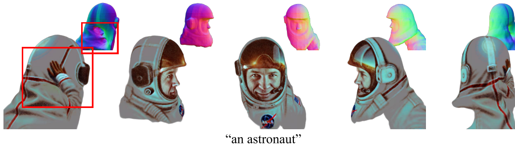
Figure 21: Hollow Face Illusion: some shapes might be generated with a concave hole in the geometry, while the rendering appears to be convex.
