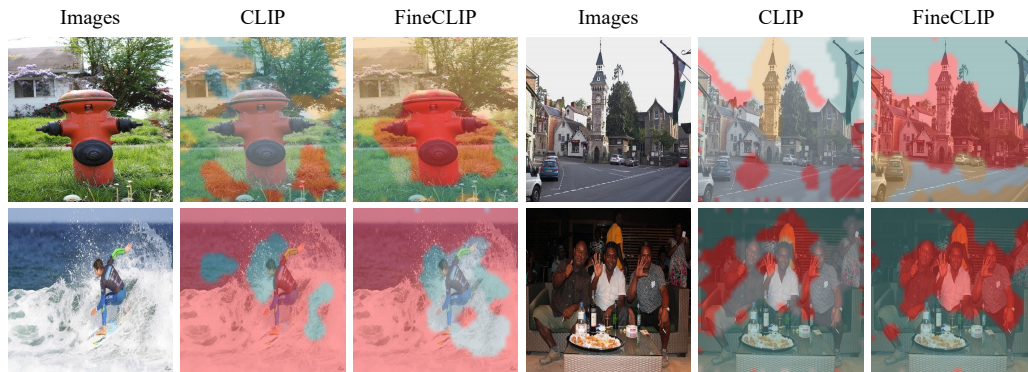
Figure 4: K-Means visualization of the dense features of CLIP ViT. We show the raw images, the K-means results of the pre-trained CLIP ViT, and those of our FineCLIP ViT.
