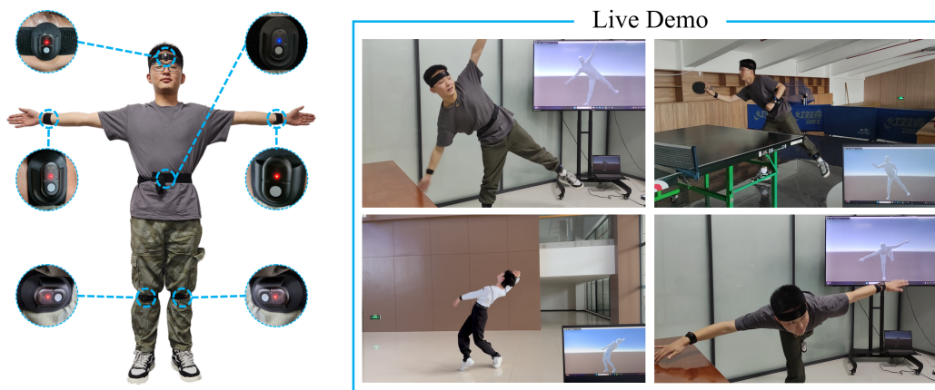
Figure 1: Left: we use only six IMUs to predict the full-body pose in real-time, which are fixed on left and right forearm, the left and right lower leg, the head, and the pelvis. Right: our system is capable of capturing a wide range of daily motions as well as challenging movements.
