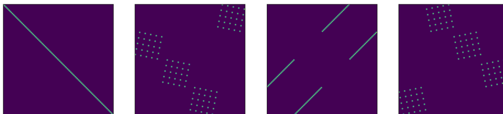
Figure 9: Ground-truth permutation matrices for C_4 rotations for 5 \times 5 spatial kernel, implementing a shift-twist operator.
