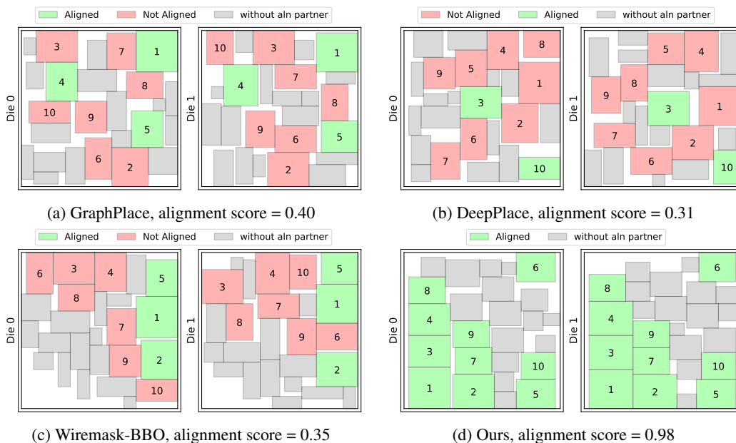
Figure 4: Visualization of cross-die block alignment on circuit n50. Two blocks with the same index forms an alignment pair. For a pair with block i, j , we calculate individual alignment score aln(i, j) according to Eq. 1. Green means these two blocks are aligned ( aln(i, j) \geq 0.5 ) while red means not aligned ( aln(i, j) < 0.5 ). Total alignment score is calculated according to Alg. 3 in Appendix G.1. It demonstrates that our method achieves much better alignment score than other baselines.
