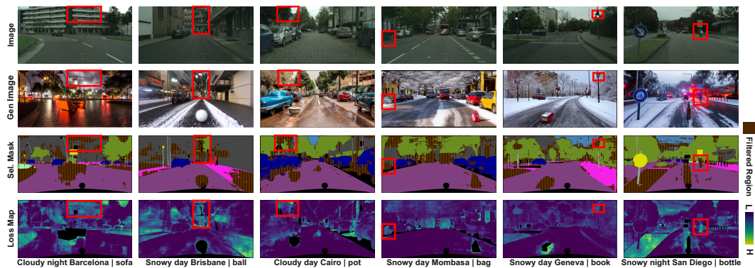
Figure 6: Visualization of Generated Images. Row 1: Original images from Cityscapes. Row 2: Generated images featuring both semantic and domain shifts. Row 3: Selection map used to calculate selected cross-entropy loss during training. Row 4: Cross-entropy loss map used to produce the selection map (excluding the OOD regions, which are not involved in known class segmentation loss calculation). Below each column, we display the weather, time, and location prompts that guide the model in generating diverse covariate shifts, along with the OOD prompts for object generation. Red boxes highlight generation errors.
