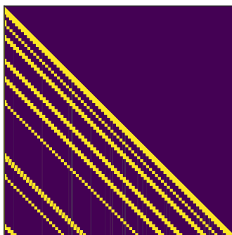
Figure 7: The dynamic sparse mask for the vertical-slash pattern using LLaMA-3-8B in the summarization task [ZCH + 24]. Yellow areas indicate the computed parts. Slash lines use 64 \times 64 blocks, while vertical lines use 1 \times 64 blocks.
