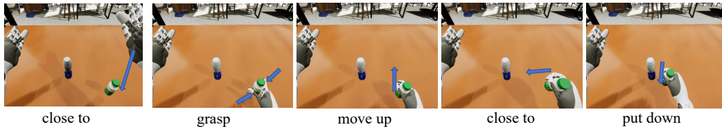
Figure 3: Examples show the execution process of PIVOT-R. The text below the image describes the primitive actions to be performed next. Blue arrows indicate the direction of actions.
