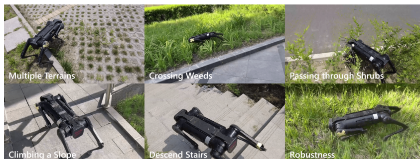
Figure 11: Real-world results for Aliengo robot with different joint failure in different terrains.
