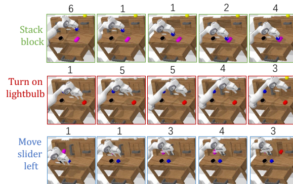
Figure 5: Visualization of DeeR rollouts in the CALVIN environment. Please zoom in to view details. The numbers indicate the termination exit index. Situations with a lower exit index are recognized as 'easier' ones.
