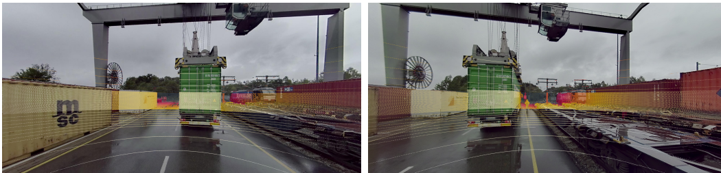
Figure A3: Projection of the left lidar sensor onto the front left camera image (left) and the right lidar sensor on the right front camera image (right). The color of the points indicates the relative distance.
