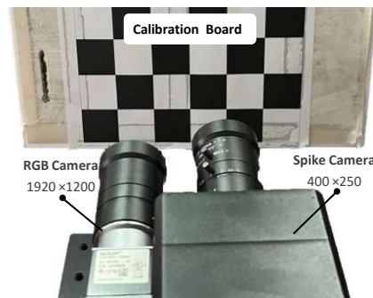
Figure 10: RGB-Spike camera system.
