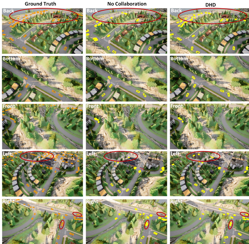
Figure 12: The visualizations illustrate the enhancement of collaborative 3D object detection in CoPerception-UAVs. For clarity, we select one of the five collaborative drones in this dataset, each equipped with five cameras. The red circles highlight areas where single-drone perception fails to detect objects, but our DHD framework successfully detects them.
