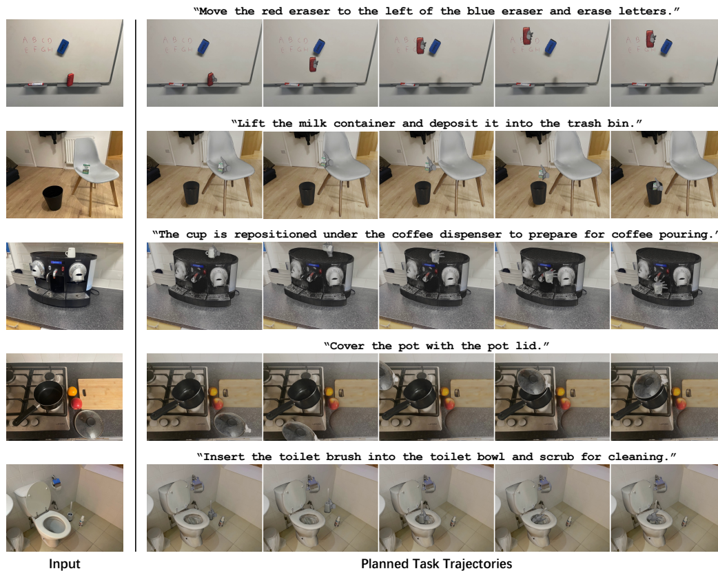
Figure 9: More qualitative examples. With diverse input scenes and proposed tasks, our framework produces 3D trajectories with geometric awareness that aligns with the task descriptions. Zoom in for better view.
