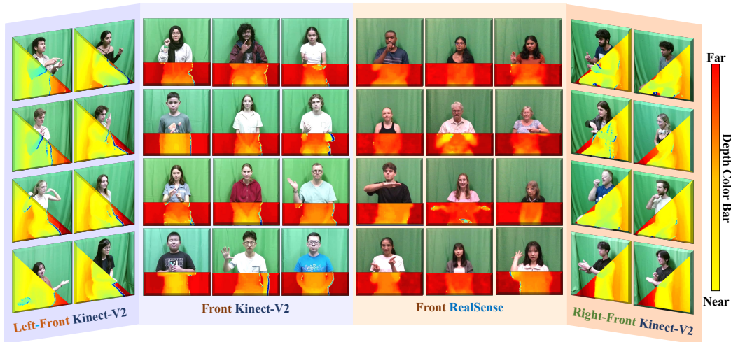
Figure 1: Illustrations of the curated MM-WLAuslan dataset. MM-WLAuslan includes three Kinect-V2 cameras and a RealSense camera arranged hemispherically around the front half of the signer to capture multi-view and multi-modal data.
