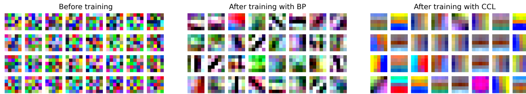
Figure 4: Visualization of the First Layer Convolutional Kernels of the Forward Model Trained with Error Backpropagation (BP) and Counter-Current Learning (CCL). Kernels from models trained with BP have more high-frequency components, as manifested as neighboring white (e.g., weight with high values) and black pixels (e.g., weight with low values). In comparison, those with CCL have more low-frequency components. We posit this might be because the error signal can contain more high-frequency information than the ideal target signal.
