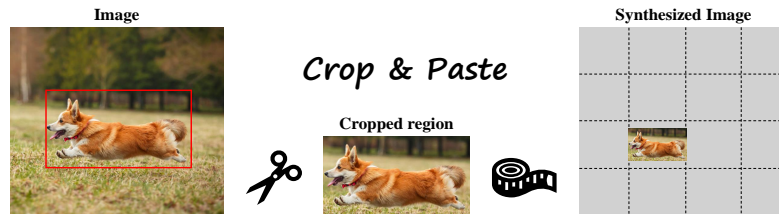
Figure 5: Workflow illustration on how we synthesize testing data. Given an image and box annotation for one object instance, we crop it and paste it on a template image, initialized with ImageNet mean pixel values. We paste every cropped region on every spatial position. Resulting data constitutes a large amount of questions about object existence, diverse in spatial positions.
