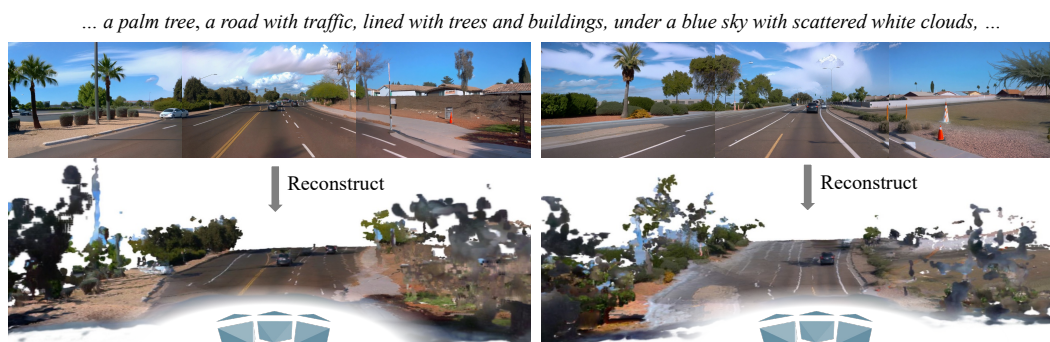
Figure 7: Text-2-Scene Generation. Given a text prompt, we could generate various multi-view images and lift them to 3D scenes with SCube. See Appendix D.3 for more text-2-scene results.
