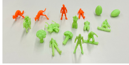
Figure 2: 3D-printed figurines created with Atlas3D stand stably, while those without Atlas3D have fallen down.
