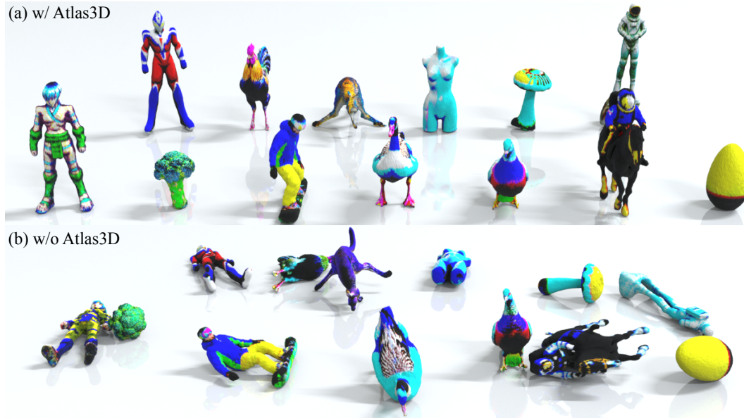
Figure 1: Simulation in ABD [27]: (a) 3D models generated from our Atlas3D framework can stand steadily on the ground; (b) those generated from existing methods tend to fall over.
