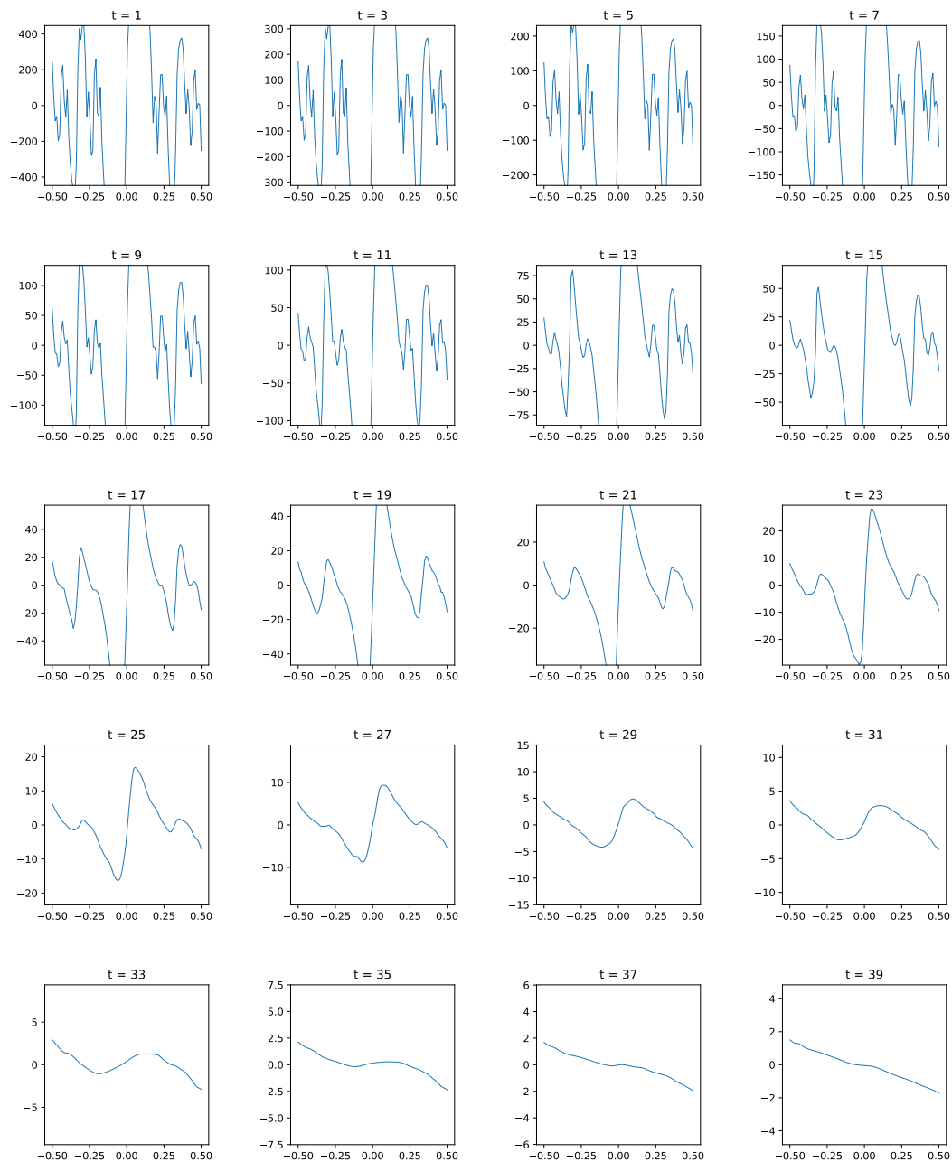
Figure 7: Evolution of the estimated score for the mollified Cantor distribution Section 4.1 with a Corrector Optimised Schedule. In this case the linear schedule fails to evenly progress the progression of the score, see Figure 6 showing the terminal score estimate in this case. The estimated score exhibits a self-similar nature of interweaving roots around the centers of mass of the mollified Cantor distribution. Identification of these roots amounts to estimated modes in our density estimate, see Figure 1.
